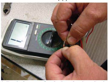
2. Test the fuse to confirm that it needs to be replaced. Any reading other than 100-500 ohms indicates a blown fuse.
