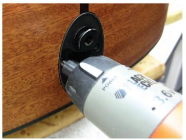
6. Re-install the power supply, plug in and test the pickup system.
