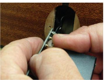
5. Insert the new fuse into the I/O board, in either direction (there is no positive or negative terminal).
