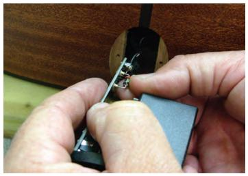
1. Remove the power supply from the tail end of the guitar (see Section VII). The fuse is located at the back end of the I/O board next to the string ground wire. It is not soldered - simply pull it out.
